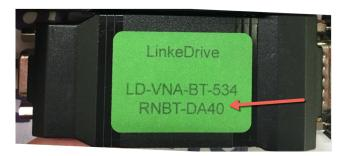
1) Make sure your VNA is securely fastened to your J1939 cable by tighting the two thumb screws. This cable can be black, or green, depending on the model and make of your tractor. Once the VNA is securely fastened, locate the diagnostic port of your tractor, and insert the J1939 cable in as shown in the right hand image. As noted, the J1939 screw clip will need to be "locked" in place; also detailed in the left hand image below.
